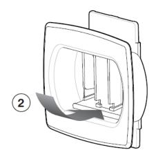
2. Continue pressing on the paddle until it rotates all the way in and locks into place.
